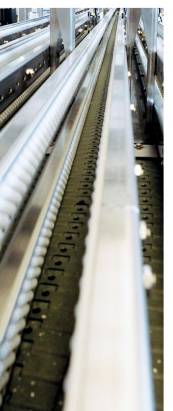
Vacuum Tech is the right solution designed and manufatured by Vetromeccanica, to convey lightweight, instable, empty containers.
